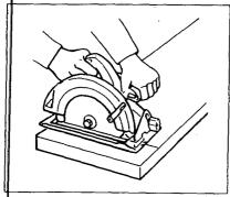
16. Never attempt to saw with the circular saw held upside down in a vise. This is extremely dangerous and can lead to serious accidents.
